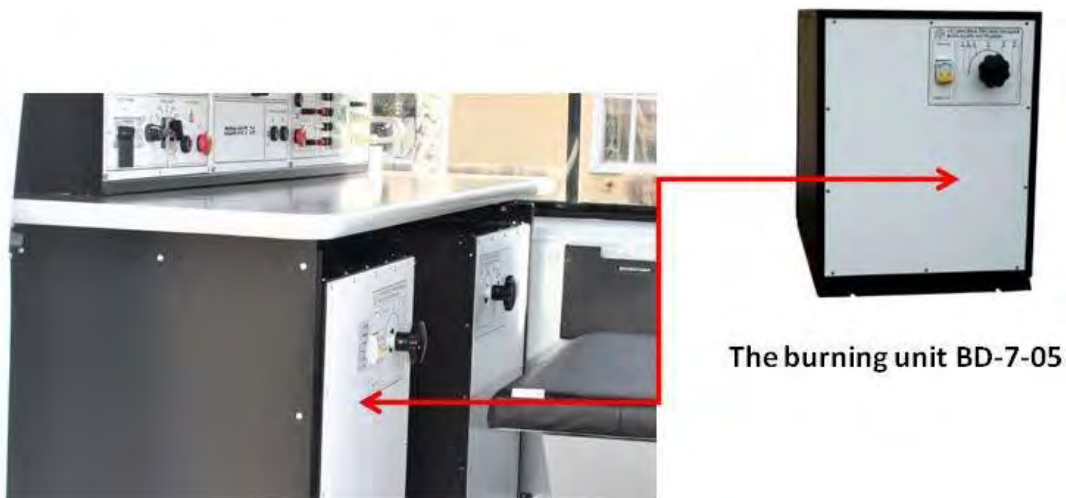
View of the Fault Burner 'BD-7-05'
