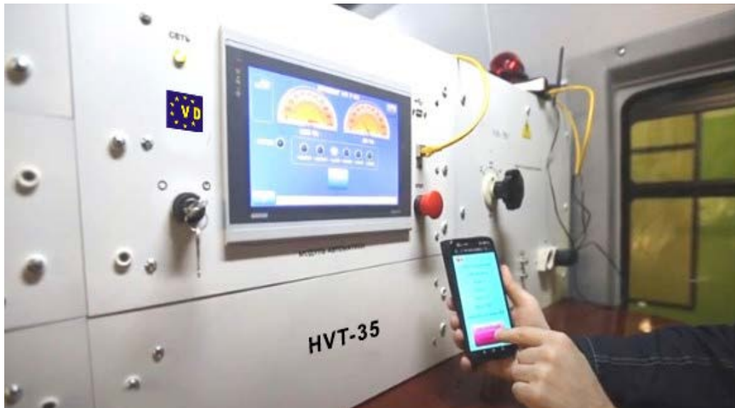
Emergency Shutdown of the laboratory remotely through a Smartphone
