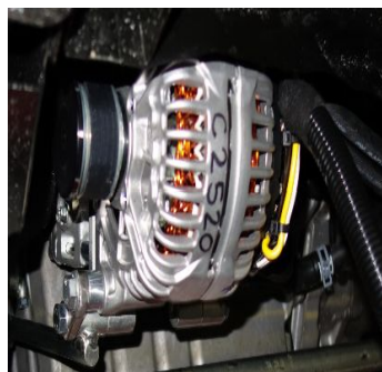
* Engine Mounted Generator
