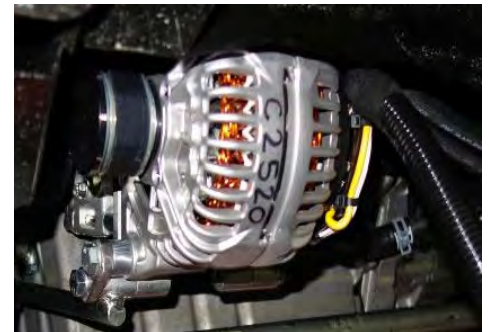
* Engine Mounted Generator
