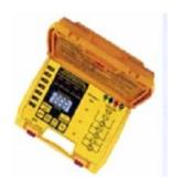
Measurement of step voltage ~U 0.01...200 V, frequency 50...60 Hz, accuracy ± 1%, Resistance 0.001 Ohm ....20 k Ohm, measurement by 2-, 3-, 4- wire scheme. Testing signal 2, 10, 50 mA, 128 Hz (allows making measurements without switching off the measuring diagram!)
