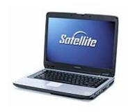
The notebook allows to store and manage the measurement data. The supplied software of the equipment is installed on the device in order to process the measurement data in the laboratory. Windows 95/98, Application package for processing of measurement results "RAD" and "POISK". Display: 15.4" WXGA (1200 x 800). Processor: Intel ® Celeron ® M 1.5 GHz.
